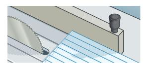
Can be cut with a fine tooth circular saw or hand saw at a shallow angle.
