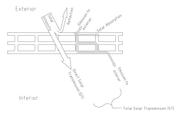
The values for direct transmission and total solar transmission are determined according to EN410 standard.
